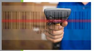
Long Range Laser scan engines offer similar functionality to laser scan engines but at a much longer range, sometimes able to read barcodes at up to 30 feet or more. If you need to
